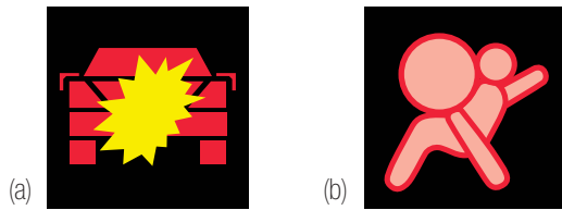
Figure 3. Sample icons for (a) forward collision warning and (b) verifying that an airbag is functional. The airbag icon is one of several symbols that the US Department of Transportation has standardized as part of efforts to arrive at a common driver-vehicle interface.
