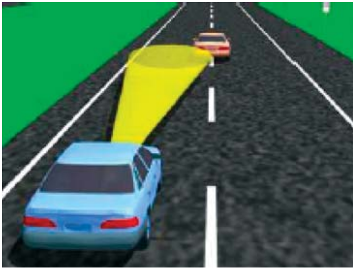
Figure 4. A forward collision warning system. Sensors detect the vehicle's proximity to other vehicles, providing data to a warning system algorithm. If the algorithm determines that the signals exceed a predetermined threshold, it activates the system to alert the driver.
