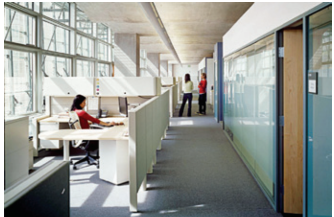
Figure 1. General Services Administration green building in San Francisco. Raised furniture and private work areas that end below the concrete ceiling enable natural light and promote airflow for more efficient heating and cooling. (Image used with permission from Roland Halbe Fotografie; www.rolandhalbe.de .)
