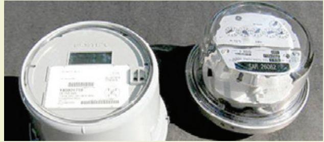
Figure A. Smart meter (left) versus a traditional meter (right). The smart meter comes with a digital readout and enables two-way communication about resource consumption, in this case water. The standard meter can only measure resources consumed and must be read. Photo used with permission from Blue Water Power; http://www.bluewaterpower.com/energyservices/Smart-Photos.html .
